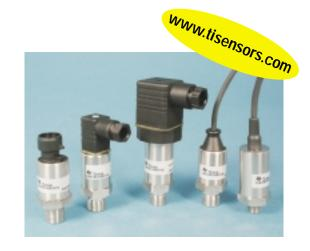
The 83HP Series is ideally suited for severe industrial OEM applications. This is a high accuracy, high level Vdc output that requires no end user amplification. Housed in corrosion resistant stainless steel, the 83HP includes a hermetic front end with a variety of electrical connectors. This transducer is available in sealed gage and vented gage from 15 psi up to 30,000 psi with several package options.
